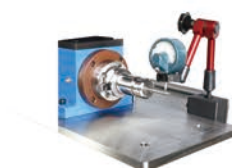
校正筒夹公差 Correction collet tolerances
