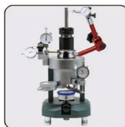
刀柄综合跳动测量 integrated runout of tool holder
